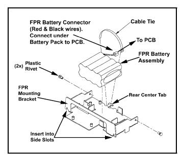
Figure 2-5. FPR & Mounting Bracket.
